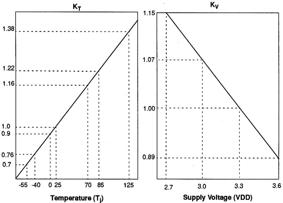
**Figure 1.1: Effect of Temperature and Supply Voltage on Propagation Delay**
